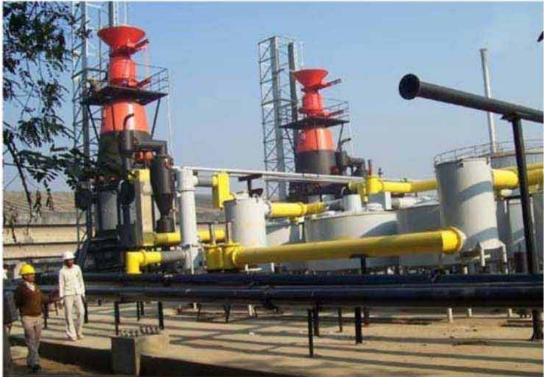
2 X WBG-1500 gasifiers for Drying Application, India
